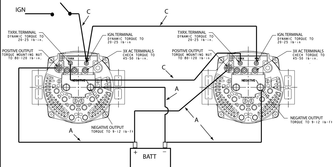
**NOTE:** Load bearing cables (A) need to be the same length and wire size, and connected to a common point. This is needed to enhance the load sharing of each alternator.
